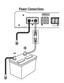
**NOTE:** It is important to upgrade the ground connection between the negative (-) battery post and the vehicle body or chassis to achieve optimum electrical performance.
